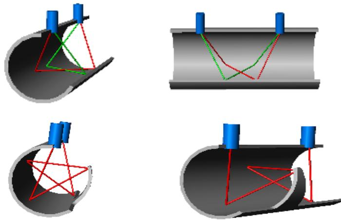
Figure 4. Variants of passing ultrasonic signals between transducers.
