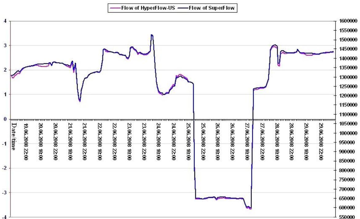
Figure 9. Diagram of flow rates, measured by ultrasonic and pressure differential flowmeters.
