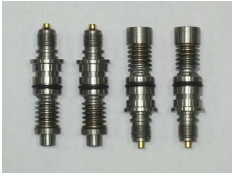
Figure 2. Piezoelectric transducers of flowmeter.
