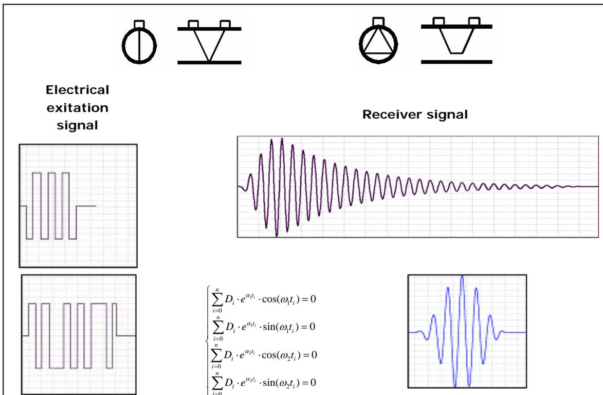
Figure 3. Formation of acoustic signal.
